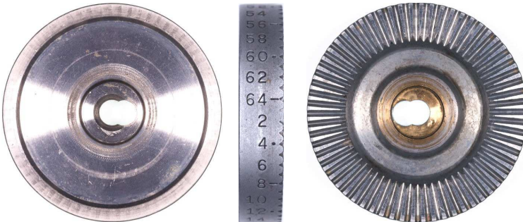
Lee Facet Head: ID OD: 1 5/8" ID: 3/8" thick: 5/16" Material: Manganese bronze (63g) or Aluminum (25g) Available in: 32,60,64,80,96
